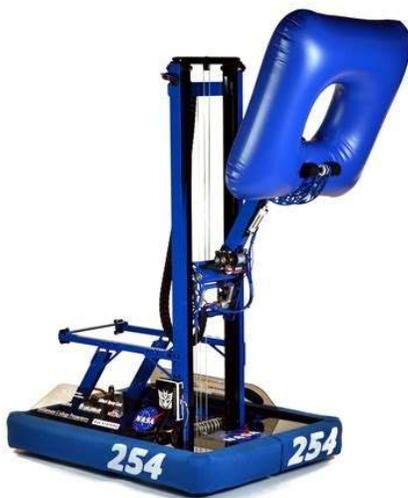
Team 254 used a belt powered system in 2011 on *Slipstream*.
