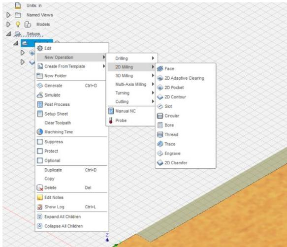
Once the contour is selected you can select the bit needed. For cutting metal and other hard materials the 1/8in bit is the one that is the best to use.
