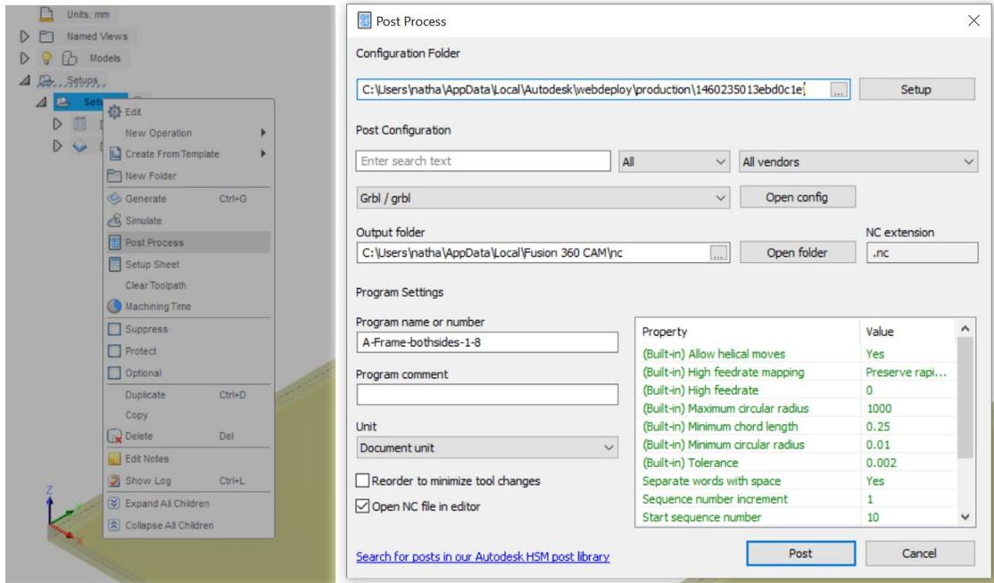
Our router runs GRBL as the Gcode language. This allows for communication between the router and the computer running the Gcode from this point when post is pressed the file output folder and name can be set. After the file goes through exports a Gcode editor will appear. We need to delete line 12 which is a command that sets the speed of the router. With our configuration this line will cause a error if left in.
