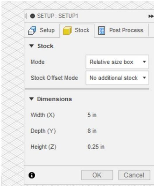
After the additional stock is removed it is important to select the origin point for the cut, we use the bottom left hand corner. Once the setup is created you can now start to create the actual cutting paths. For the majority of cuts needed the contour tool is the one that you need to use.
