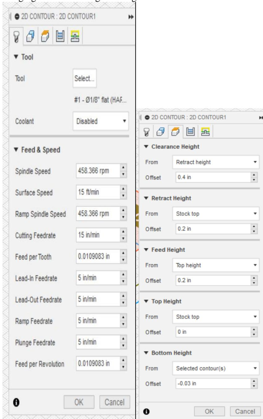
This is important due to the fact that the thickness of the material is often not the same size that is shown in CAD. Before exiting the contour creation box it is necessary to change the number of depths that the bit goes through before reaching the bottom of the material. For metal 10 thousands of an inch is normally standard. For other materials it is best to search online and use good judgment to find the right cutting depth.
