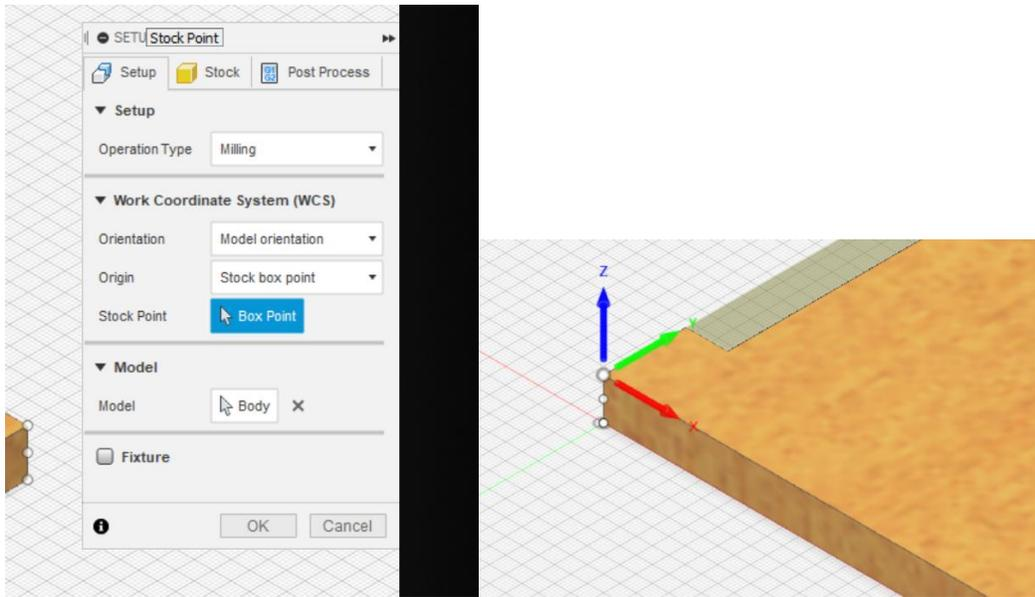
Be sure the Z and X axis are set correctly. While still in the setup screen be sure to select no additional stock under the stock tab.
